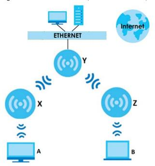
The following figure shows an example of a wireless bridge network. The root AP (Y) is connected to a network with Internet access and has a wireless repeater (X) connected to it to expand the wireless network's range. Clients (A and B) are connected to the wired network through the gateway (G). They can access the wired network through the wireless repeater and/or root AP.
