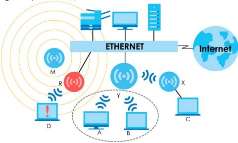
The following figure shows you how to create a secure Wireless Distribution System (WDS). The root AP (Y) is connected to a network with Internet access and has wireless repeaters (X and Z) connected to it to expand the wireless network's range. Clients (A and B) can access the wired network through the wireless repeaters (X and Z) and/or root AP.
